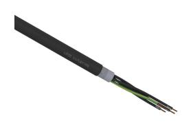
LUTZE Silflex FBP flexible control cable, shielded, 5 conductors (includes ground), 14 AWG, bare copper, polypropylene conductor insulation material, black with white numbers and green/yellow ground, TPE jacket, black, cut to length.
