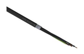
LUTZE Silflex FBP flexible control cable, shielded, 4 conductors (includes ground), 14 AWG, bare copper, polypropylene conductor insulation material, black with white numbers and green/yellow ground, TPE jacket, black, cut to length.
