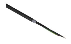
LUTZE Silflex FBP flexible control cable, shielded, 3 conductors (includes ground), 14 AWG, bare copper, polypropylene conductor insulation material, black with white numbers and green/yellow ground, TPE jacket, black, cut to length.
