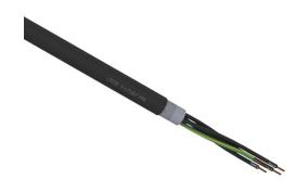
LUTZE Silflex FBP flexible control cable, shielded, 5 conductors (includes ground), 12 AWG, bare copper, polypropylene conductor insulation material, black with white numbers and green/yellow ground, TPE jacket, black, cut to length.
