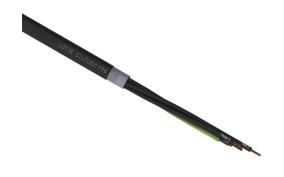
LUTZE Silflex FBP flexible control cable, shielded, 4 conductors (includes ground), 12 AWG, bare copper, polypropylene conductor insulation material, black with white numbers and green/yellow ground, TPE jacket, black, cut to length.
