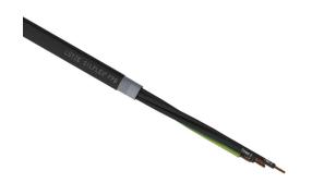
LUTZE Silflex FBP flexible control cable, shielded, 4 conductors (includes ground), 10 AWG, bare copper, polypropylene conductor insulation material, black with white numbers and green/yellow ground, TPE jacket, black, cut to length.
