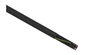
LUTZE Silflex FBP flexible control cable, unshielded, 25 conductors (includes ground), 20 AWG, bare copper, polypropylene conductor insulation material, black with white numbers and green/yellow ground, TPE jacket, black, cut to length.
