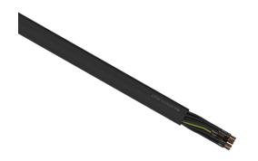
LUTZE Silflex FBP flexible control cable, unshielded, 18 conductors (includes ground), 20 AWG, bare copper, polypropylene conductor insulation material, black with white numbers and green/yellow ground, TPE jacket, black, cut to length.
