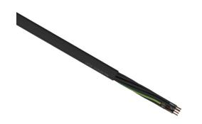
LUTZE Silflex FBP flexible control cable, unshielded, 12 conductors (includes ground), 20 AWG, bare copper, polypropylene conductor insulation material, black with white numbers and green/yellow ground, TPE jacket, black, cut to length.
