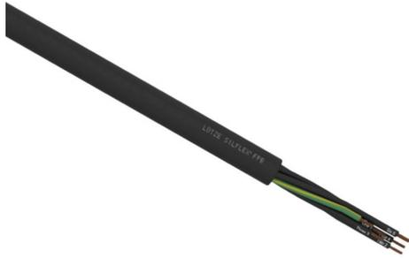
LUTZE Silflex FBP flexible control cable, unshielded, 7 conductors (includes ground), 20 AWG, bare copper, polypropylene conductor insulation material, black with white numbers and green/yellow ground, TPE jacket, black, cut to length.
