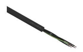
LUTZE Silflex FBP flexible control cable, unshielded, 5 conductors (includes ground), 20 AWG, bare copper, polypropylene conductor insulation material, black with white numbers and green/yellow ground, TPE jacket, black, cut to length.
