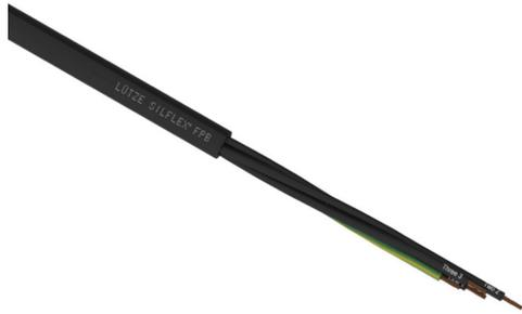
LUTZE Silflex FBP flexible control cable, unshielded, 4 conductors (includes ground), 20 AWG, bare copper, polypropylene conductor insulation material, black with white numbers and green/yellow ground, TPE jacket, black, cut to length.
