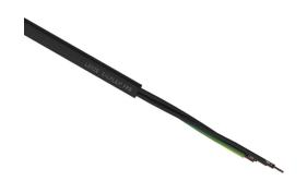
LUTZE Silflex FBP flexible control cable, unshielded, 3 conductors (includes ground), 20 AWG, bare copper, polypropylene conductor insulation material, black with white numbers and green/yellow ground, TPE jacket, black, cut to length.
