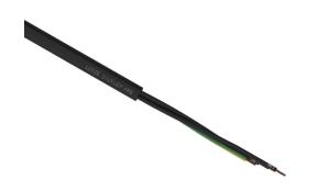
LUTZE Silflex FBP flexible control cable, unshielded, 3 conductors (includes ground), 20 AWG, bare copper, polypropylene conductor insulation material, black with white numbers and green/yellow ground, TPE jacket, black, cut to length.
