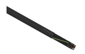
LUTZE Silflex FBP flexible control cable, unshielded, 25 conductors (includes ground), 18 AWG, bare copper, polypropylene conductor insulation material, black with white numbers and green/yellow ground, TPE jacket, black, cut to length.
