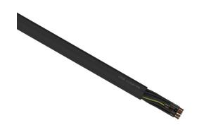
LUTZE Silflex FBP flexible control cable, unshielded, 18 conductors (includes ground), 18 AWG, bare copper, polypropylene conductor insulation material, black with white numbers and green/yellow ground, TPE jacket, black, cut to length.
