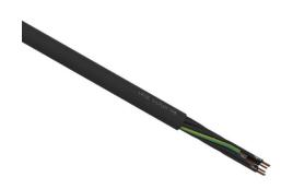
LUTZE Silflex FBP flexible control cable, unshielded, 9 conductors (includes ground), 18 AWG, bare copper, polypropylene conductor insulation material, black with white numbers and green/yellow ground, TPE jacket, black, cut to length.
