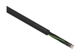
LUTZE Silflex FBP flexible control cable, unshielded, 7 conductors (includes ground), 18 AWG, bare copper, polypropylene conductor insulation material, black with white numbers and green/yellow ground, TPE jacket, black, cut to length.
