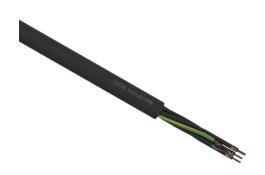
LUTZE Silflex FBP flexible control cable, unshielded, 7 conductors (includes ground), 18 AWG, bare copper, polypropylene conductor insulation material, black with white numbers and green/yellow ground, TPE jacket, black, cut to length.
