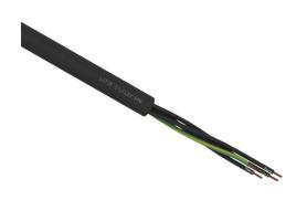
LUTZE Silflex FBP flexible control cable, unshielded, 5 conductors (includes ground), 18 AWG, bare copper, polypropylene conductor insulation material, black with white numbers and green/yellow ground, TPE jacket, black, cut to length.
