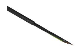
LUTZE Silflex FBP flexible control cable, unshielded, 4 conductors (includes ground), 18 AWG, bare copper, polypropylene conductor insulation material, black with white numbers and green/yellow ground, TPE jacket, black, cut to length.
