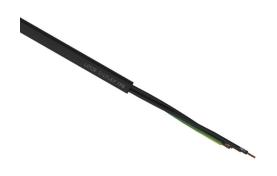
LUTZE Silflex FBP flexible control cable, unshielded, 3 conductors (includes ground), 18 AWG, bare copper, polypropylene conductor insulation material, black with white numbers and green/yellow ground, TPE jacket, black, cut to length.
