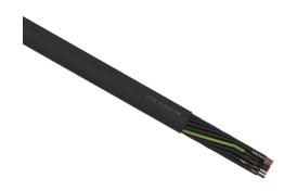
LUTZE Silflex FBP flexible control cable, unshielded, 25 conductors (includes ground), 16 AWG, bare copper, polypropylene conductor insulation material, black with white numbers and green/yellow ground, TPE jacket, black, cut to length.
