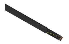
LUTZE Silflex FBP flexible control cable, unshielded, 18 conductors (includes ground), 16 AWG, bare copper, polypropylene conductor insulation material, black with white numbers and green/yellow ground, TPE jacket, black, cut to length.
