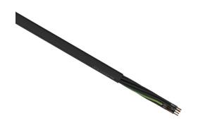
LUTZE Silflex FBP flexible control cable, unshielded, 12 conductors (includes ground), 16 AWG, bare copper, polypropylene conductor insulation material, black with white numbers and green/yellow ground, TPE jacket, black, cut to length.
