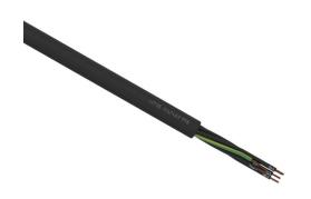
LUTZE Silflex FBP flexible control cable, unshielded, 7 conductors (includes ground), 16 AWG, bare copper, polypropylene conductor insulation material, black with white numbers and green/yellow ground, TPE jacket, black, cut to length.
