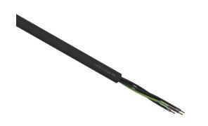
LUTZE Silflex FBP flexible control cable, unshielded, 5 conductors (includes ground), 16 AWG, bare copper, polypropylene conductor insulation material, black with white numbers and green/yellow ground, TPE jacket, black, cut to length.
