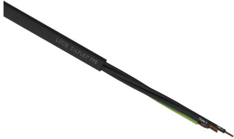
LUTZE Silflex FBP flexible control cable, unshielded, 4 conductors (includes ground), 16 AWG, bare copper, polypropylene conductor insulation material, black with white numbers and green/yellow ground, TPE jacket, black, cut to length.
