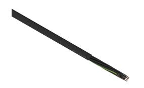
LUTZE Silflex FBP flexible control cable, unshielded, 12 conductors (includes ground), 14 AWG, bare copper, polypropylene conductor insulation material, black with white numbers and green/yellow ground, TPE jacket, black, cut to length.
