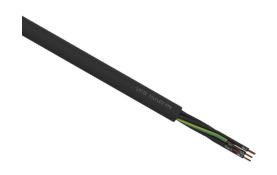
LUTZE Silflex FBP flexible control cable, unshielded, 7 conductors (includes ground), 14 AWG, bare copper, polypropylene conductor insulation material, black with white numbers and green/yellow ground, TPE jacket, black, cut to length.
