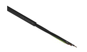
LUTZE Silflex FBP flexible control cable, unshielded, 4 conductors (includes ground), 14 AWG, bare copper, polypropylene conductor insulation material, black with white numbers and green/yellow ground, TPE jacket, black, cut to length.
