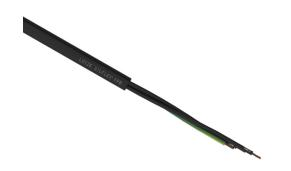
LUTZE Silflex FBP flexible control cable, unshielded, 3 conductors (includes ground), 14 AWG, bare copper, polypropylene conductor insulation material, black with white numbers and green/yellow ground, TPE jacket, black, cut to length.
