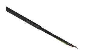
LUTZE Silflex FBP flexible control cable, unshielded, 4 conductors (includes ground), 12 AWG, bare copper, polypropylene conductor insulation material, black with white numbers and green/yellow ground, TPE jacket, black, cut to length.
