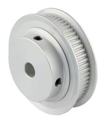
Sung-II Machinery timing pulley, aluminum, 0.08in MXL pitch, 60 tooth, 1.528in pitch diameter, 1/4in bore, hub with flanges. For use with 1/4in wide belt.
