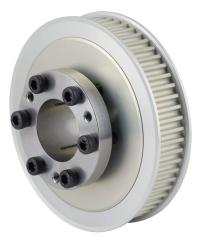
Sung-Il Machinery timing pulley, aluminum, 5mm 5M pitch, 60 tooth, 3.76in pitch diameter, 1-1/8in bore, no hub with flanges. For use with 15mm wide belt. QD bushing included.
