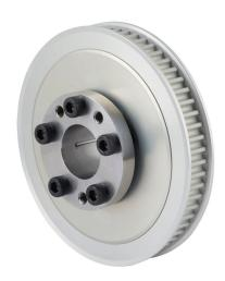
Sung-II Machinery timing pulley, aluminum, 5mm 5M pitch, 60 tooth, 3.76in pitch diameter, 7/8in bore, no hub with flanges. For use with 9mm wide belt. QD bushing included.
