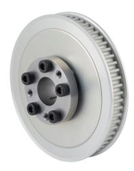
Sung-II Machinery timing pulley, aluminum, 5mm 5M pitch, 60 tooth, 3.76in pitch diameter, 3/4in bore, no hub with flanges. For use with 9mm wide belt. QD bushing included.
