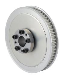
Sung-II Machinery timing pulley, aluminum, 5mm 5M pitch, 60 tooth, 3.76in pitch diameter, 5/8in bore, no hub with flanges. For use with 9mm wide belt. QD bushing included.
