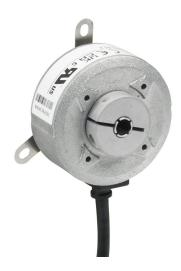
Lika Electronic A50 series incremental (quadrature) rotary encoder, medium duty, 5-30 VDC, radial exit, universal (line driver or NPN/PNP open collector) output, 1000 ppr, 1/4in hollow shaft, 50mm diameter body, IP65, 6.5ft/2m cable length, pigtail.
