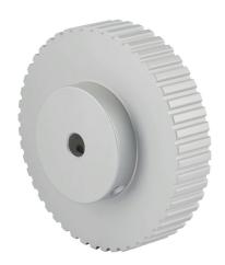
Sung-II Machinery timing pulley, aluminum, 1/5in XL pitch, 48 tooth, 3.056in pitch diameter, 5/16in bore, hub without flanges. For use with 3/8in wide belt.
