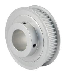
Sung-II Machinery timing pulley, aluminum, 5mm 5M pitch, 48 tooth, 3.008in pitch diameter, 1-1/8in bore, hub with flanges. For use with 15mm wide belt.
