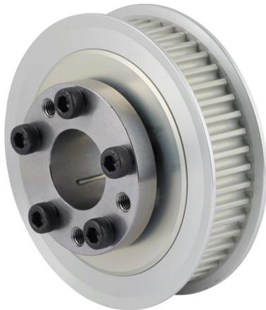
Sung-II Machinery timing pulley, aluminum, 5mm 5M pitch, 48 tooth, 3.008in pitch diameter, 7/8in bore, no hub with flanges. For use with 15mm wide belt. QD bushing included.
