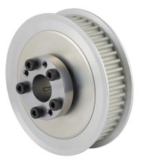
Sung-Il Machinery timing pulley, aluminum, 5mm 5M pitch, 48 tooth, 3.008in pitch diameter, 5/8in bore, no hub with flanges. For use with 15mm wide belt. QD bushing included.
