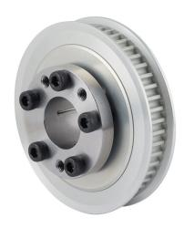
Sung-Il Machinery timing pulley, aluminum, 5mm 5M pitch, 48 tooth, 3.008in pitch diameter, 7/8in bore, no hub with flanges. For use with 9mm wide belt. QD bushing included.
