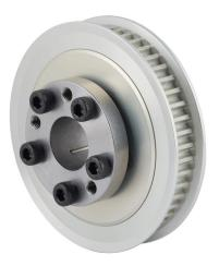
Sung-Il Machinery timing pulley, aluminum, 5mm 5M pitch, 48 tooth, 3.008in pitch diameter, 3/4in bore, no hub with flanges. For use with 9mm wide belt. QD bushing included.
