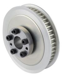
Sung-Il Machinery timing pulley, aluminum, 5mm 5M pitch, 48 tooth, 3.008in pitch diameter, 5/8in bore, no hub with flanges. For use with 9mm wide belt. QD bushing included.
