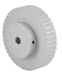
Sung-Il Machinery timing pulley, aluminum, 1/5in XL pitch, 44 tooth, 2.801in pitch diameter, 5/16in bore, hub without flanges. For use with 3/8in wide belt.
