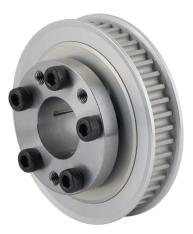
Sung-Il Machinery timing pulley, aluminum, 5mm 5M pitch, 44 tooth, 2.757in pitch diameter, 7/8in bore, no hub with flanges. For use with 9mm wide belt. QD bushing included.
