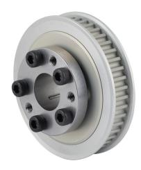
Sung-Il Machinery timing pulley, aluminum, 5mm 5M pitch, 44 tooth, 2.757in pitch diameter, 3/4in bore, no hub with flanges. For use with 9mm wide belt. QD bushing included.
