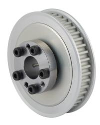
Sung-Il Machinery timing pulley, aluminum, 5mm 5M pitch, 44 tooth, 2.757in pitch diameter, 5/8in bore, no hub with flanges. For use with 9mm wide belt. QD bushing included.
