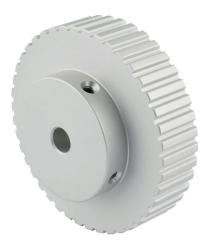
Sung-Il Machinery timing pulley, aluminum, 1/5in XL pitch, 42 tooth, 2.674in pitch diameter, 5/16in bore, hub without flanges. For use with 3/8in wide belt.
