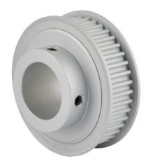
Sung-II Machinery timing pulley, aluminum, 5mm 5M pitch, 42 tooth, 2.632in pitch diameter, 1-1/8in bore, hub with flanges. For use with 15mm wide belt.
